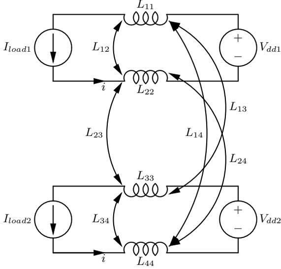
**Figure 3: Circuit diagram of the mutual inductive coupling of the proposed power distribution grid.  $L_{11}$  and  $L_{33}$  denote the partial self inductances of the power lines and  $L_{22}$  and  $L_{44}$  denote the partial self inductances of the ground lines, respectively.**
