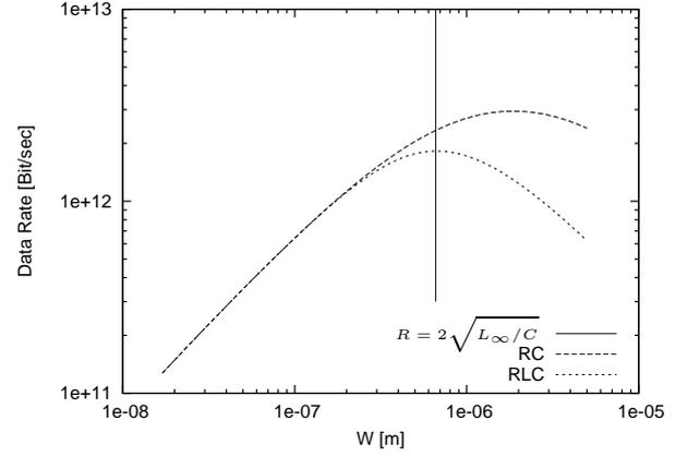
Figure 6: RC and RLC data rate vs. wires width for  $S=W$ . Solid line shows the boundary between RC and RLC models.
