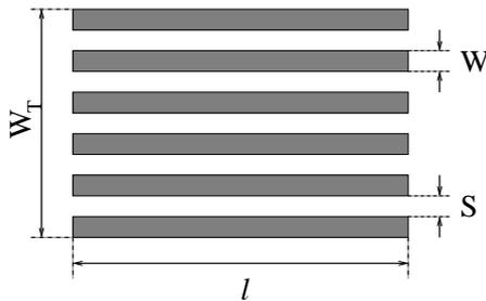
Figure 1: Link layout in an area of total width  $W_T$  and length  $l$ .  $W$  and  $S$  are wire width and spacing.
