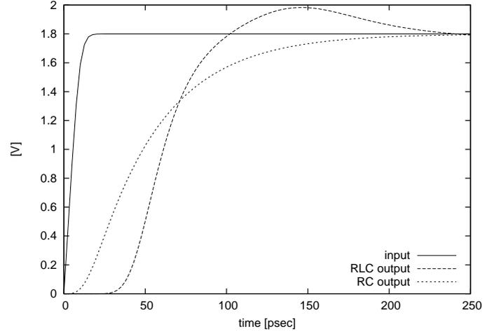
Figure 4: Simulated output waveforms using RC and RLC link models. The 50% delay is longer in the RLC model, while the signal rise time is shorter.
