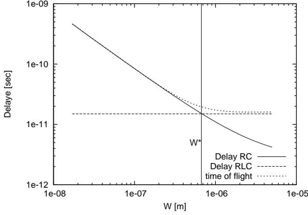
Figure 5: RC, RLC delay and time of flight vs. wires width for  $S=W$ .  $T=H=1\mu$ ,  $l=2\text{mm}$ .
