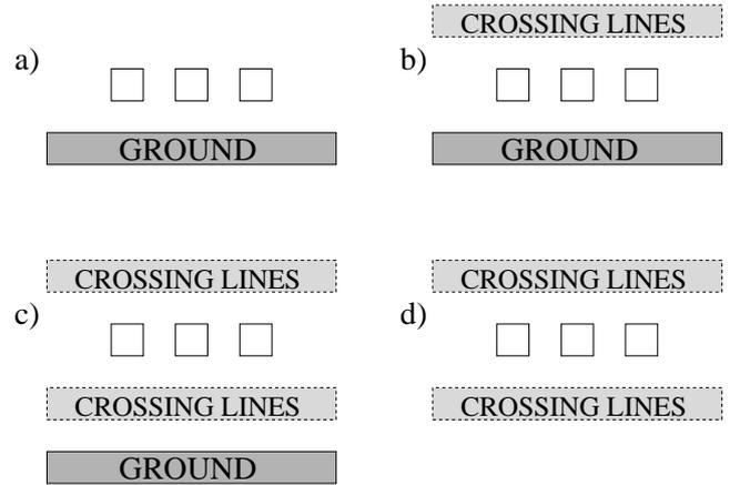
Figure 7: General link cross section: a) basic structure, b) structure with crossing lines above the link signal layer, c) structure crossing lines underneath the link signal layer, d) coplanar structure with crossing lines above and below the link
