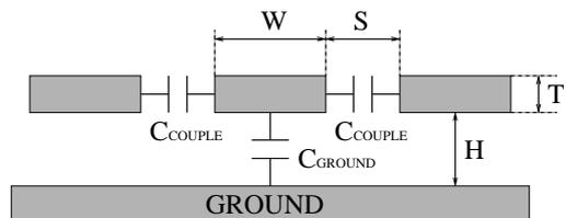
Figure 2: Basic link cross section. A solid ground plane resides under the signal lines, to ensure the current return path.
