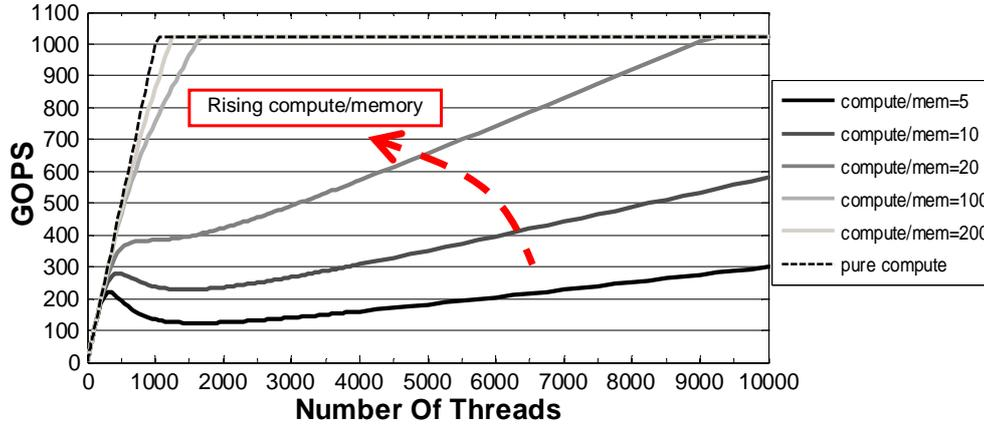
**Fig. 3. Performance for different compute/memory ratios.**
