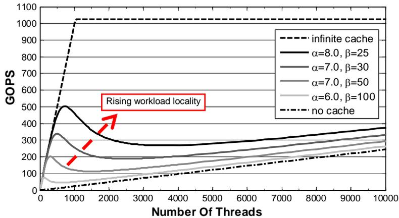
Fig. 2. Performance for different cache hit rate functions.
