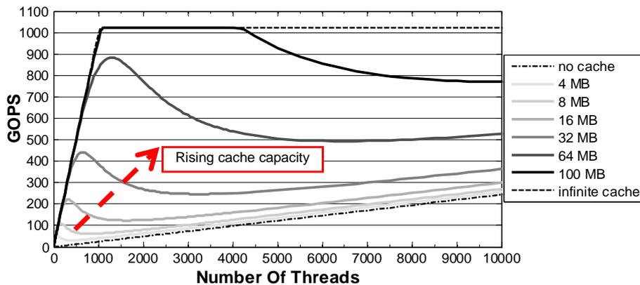
Fig. 5. Performance for different cache sizes.
