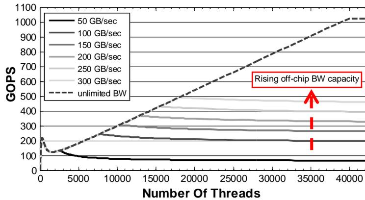
Fig. 6. Performance with limited off-chip bandwidth.
