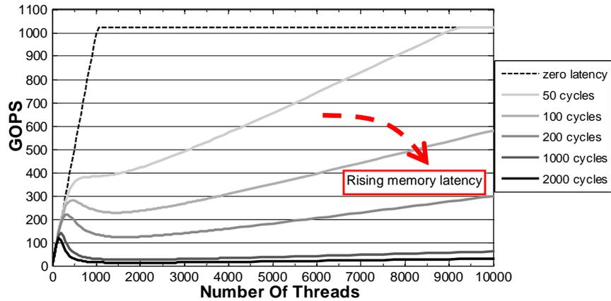
Fig. 4. Performance for different off-chip latencies.
