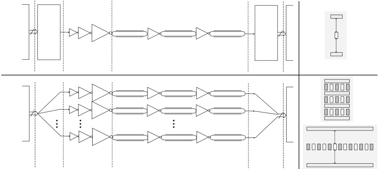
Figure 1. Serial and Parallel link architectures, related parameters and wire structures.
