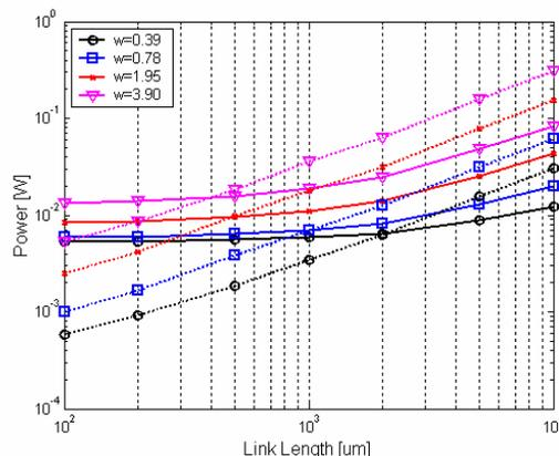
Figure 2. Power in serial and parallel links (130nm, multi-layer)
