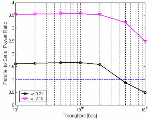
**Figure 5.** Ratio of power vs. throughput (70nm, multi-layer)
