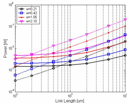
Figure 3. Power in serial and parallel links (70nm, multi-layer)
