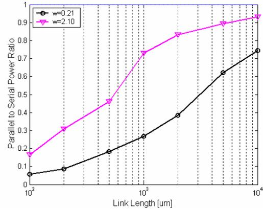
**Figure 7.** Ratio of power vs. link length (70nm, single-layer)
