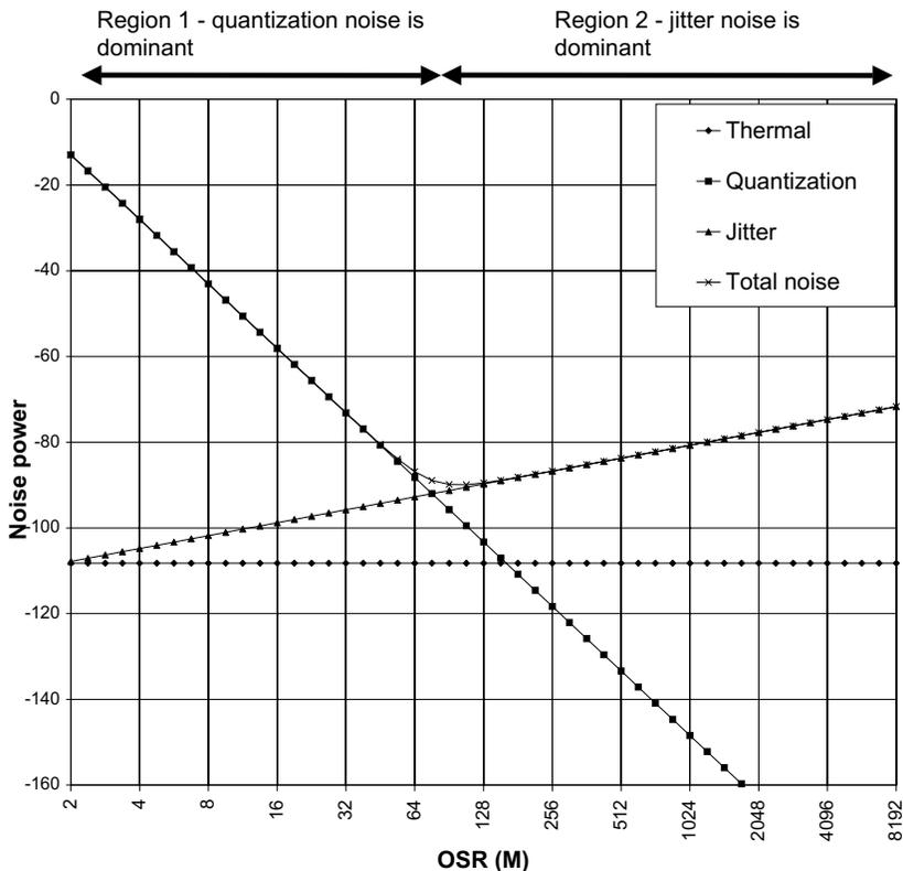
Fig. 8. Noise components in second-order continuous-time modulators. Clock jitter noise is dominant and it grows with increasing frequency. The minimum-noise point can be improved by using a low oversampling rate and a higher-order integration to further reduce quantization noise.
