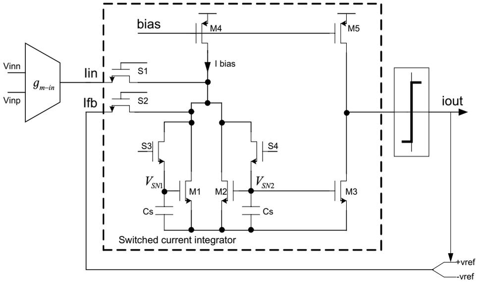
Fig. 2. Switched current modulator. Sampling capacitors  $C_S$  are MOS transistor gate capacitances.
