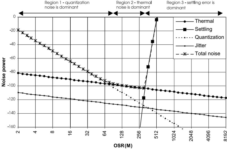
Fig. 6. Noise components in a second-order switched-capacitor sigma-delta modulator as a function of the oversampling ratio  $M$ . Thermally limited operation is achieved in the middle region ( $128 < M < 256$ ); settling noise becomes dominant at higher sampling frequencies.
