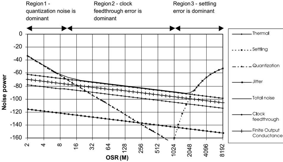
Fig. 7. Noise components in second-order switched current circuit topology. Clock feed-through and finite output conductance error dominate at middle frequencies. The useful range of oversampling ratio is limited by settling error.
