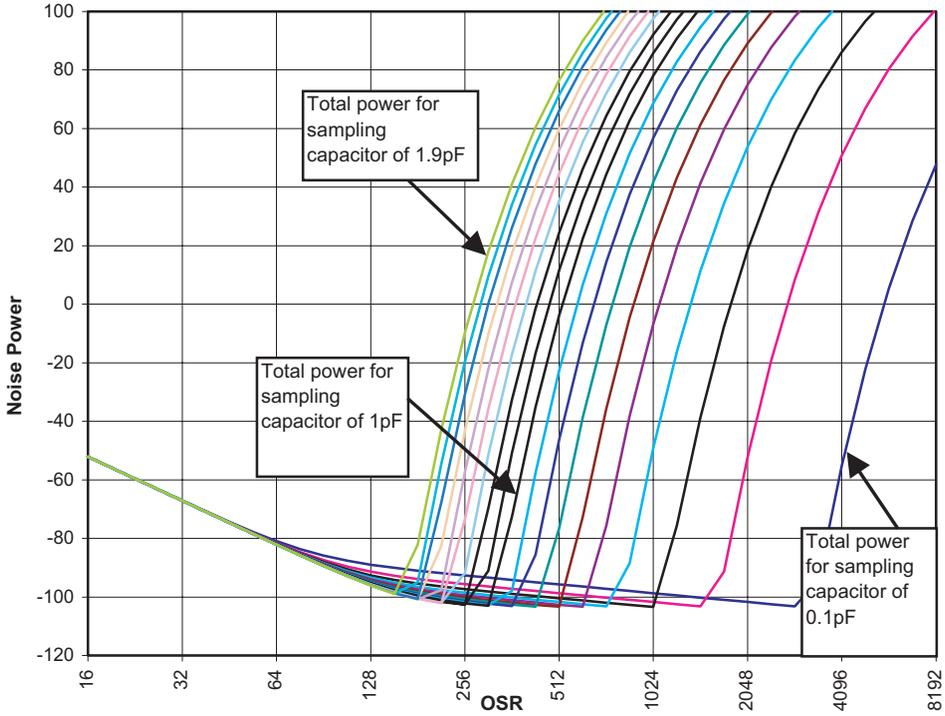
Fig. 9. Total noise power of switched capacitor sigma–delta modulator, for sampling capacitor values from 0.1 pF to 1.9 pF in 0.1 pF steps. The minimum achievable noise power is independent of the selected value of sampling capacitor.
