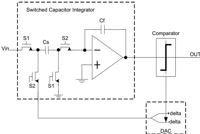
Fig. 1. First-order single-ended switched capacitor sigma-delta modulator. Sampling capacitor  $C_S$  is a linear floating capacitance.
