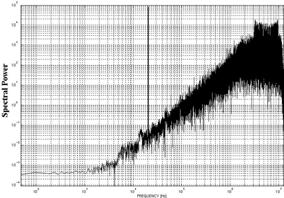
Fig. 5. Power density of a second-order sigma–delta modulator with sinusoidal input at 20 kHz, obtained from time-domain behavioral simulation, converted by FFT. The model accounts for shaped quantization noise, integrator leakage, comparator offset and output saturation. Oversampling ratio is 256, the extracted signal-to-noise ratio is  $\text{SNR} = 101$  dB assuming an ideal digital low-pass filter.
