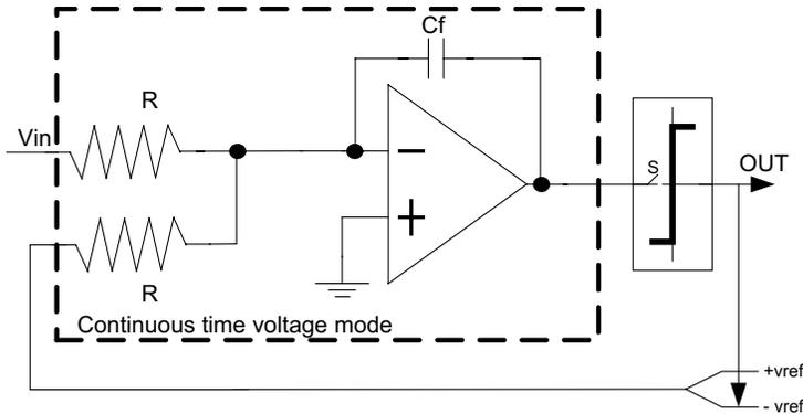
Fig. 3. Continuous time voltage mode modulator. Sampling is performed in the quantizer.
