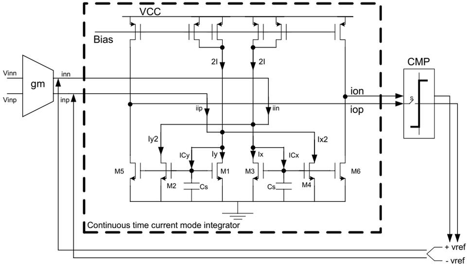
Fig. 4. Continuous time current mode modulator. A differential sampling quantizer is used.
