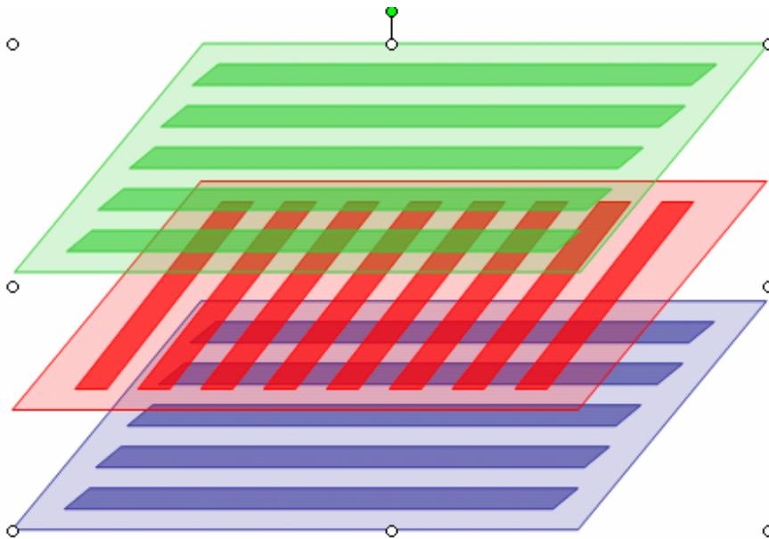
Figure 1: The interconnecting metal layer regime in VLSI chips. Metal layers are stacked one above the other and directions of interconnects are alternating between adjacent layers.
