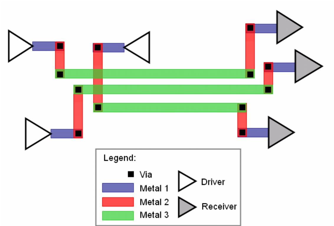
Figure 2: Interconnecting circuits in VLSI chips. A driving circuit is connected at the near end of a network. The signal is propagating along metal wires to the receiving circuit connected at the far end of the network.
