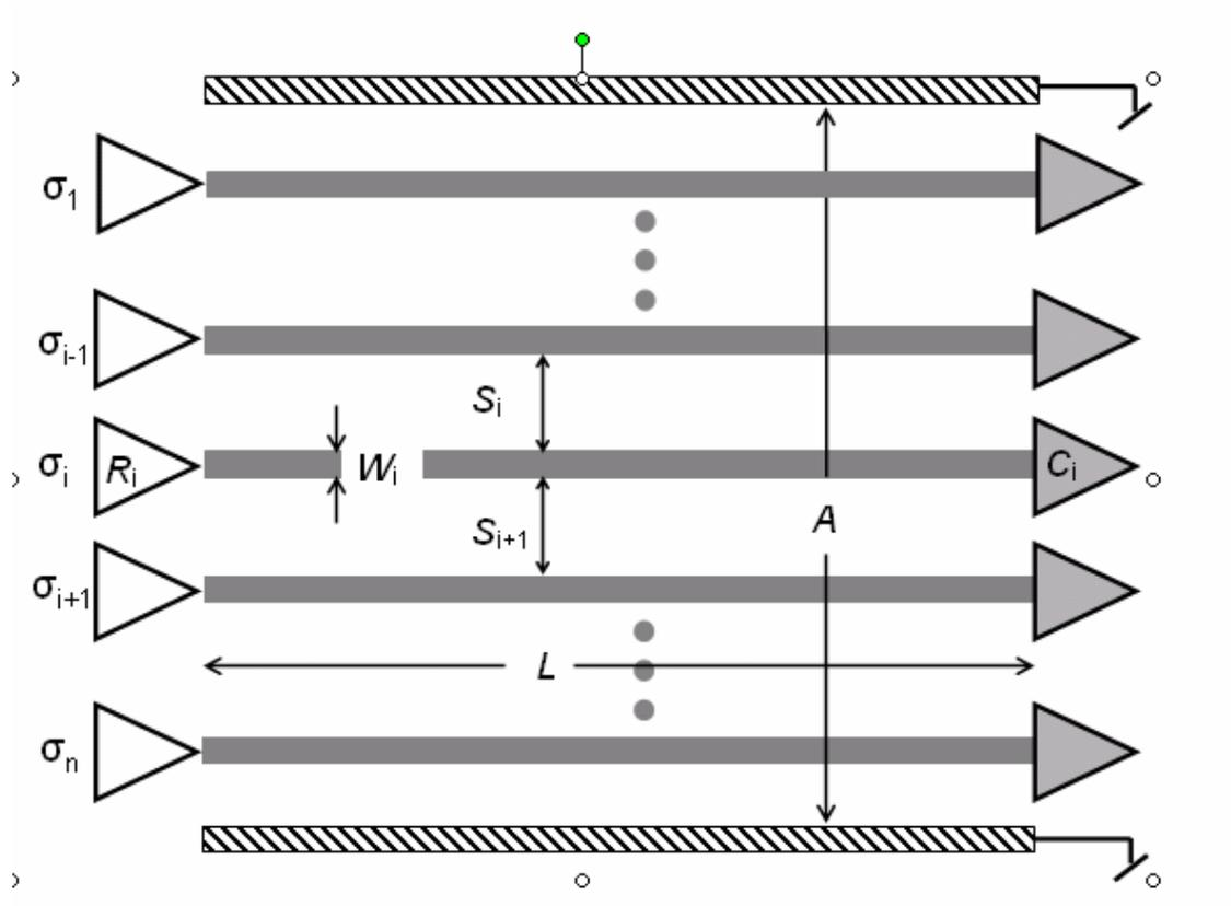
Figure 3: A fundamental model of interconnecting bus comprising parallel wires laid on the same layer between two shielding wires.
