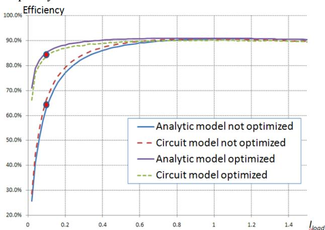
Figure 5: Optimized and non-optimized simulated vs analytic efficiency
