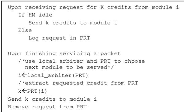
**Figure 5: Operation of a simple HM allocation controller.**
