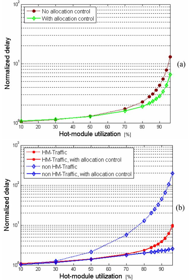
**Figure 12: Mean end-to-end delay vs. hot-modules load.**
