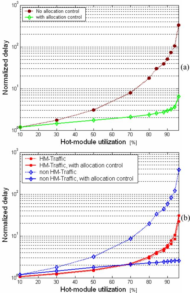
Figure 6: Mean end-to-end delay vs. HM load.
