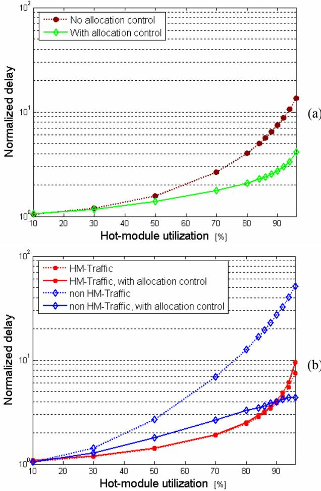
**Figure 11: Mean end-to-end delay vs. hot-modules load.**
