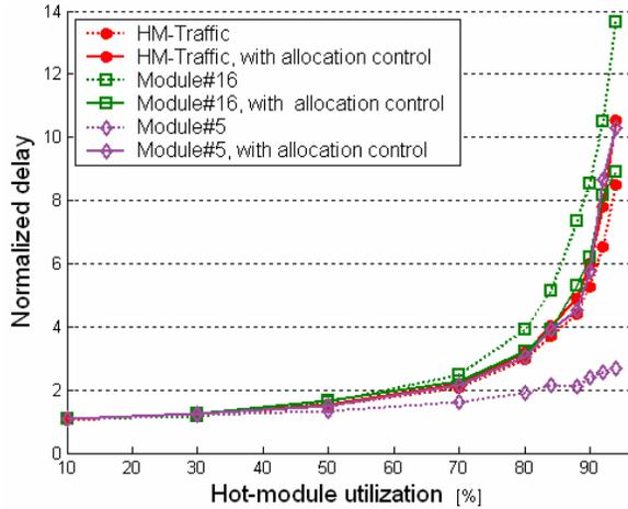
**Figure 7: Mean end-to-end delays vs. HM load.**
