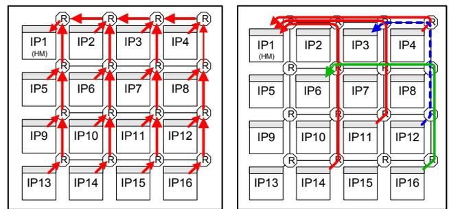
**Figure 2: Hot-module effects in a 4x4 YX routed NoC**
