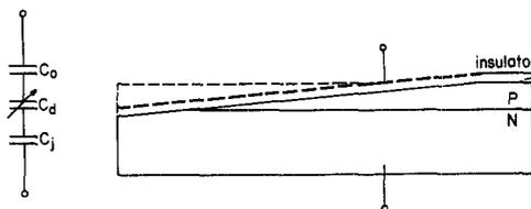
Fig. 1. Schematic cross section of a diffused sample after gradual etching and capacitor fabrication. Also shown is the capacitance model.
