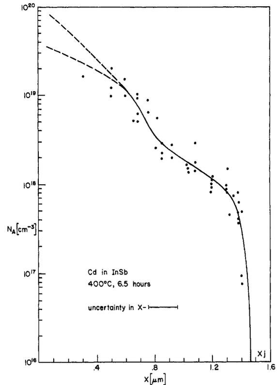
Fig. 2. Diffusion profile of Cd in InSb, measured by the graded  $C(V)$  method at 77 K. The uncertainty in the measured value of  $x$  is also indicated.
