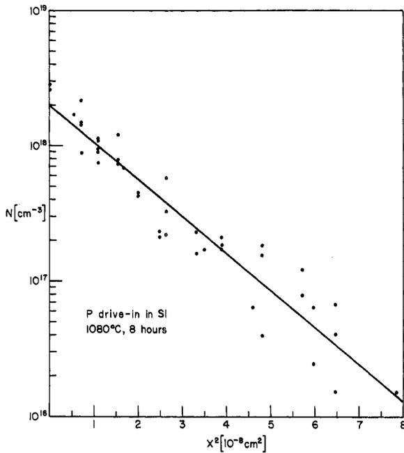
Fig. 3. Concentrations of implanted phosphorus in silicon measured by the graded  $C(V)$  method after drive-in diffusion, plotted versus squared depth. The slope of the straight line corresponds to  $D = 1.4 \times 10^{-13} \text{ cm}^2/\text{s}$ .
