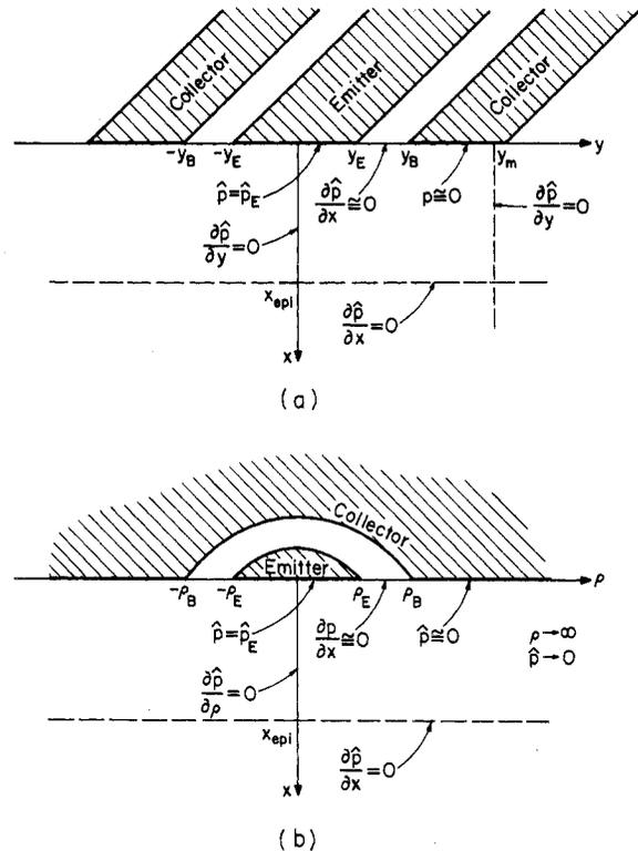
Fig. 1. Schematic view of lateral p-n-p transistors with mesa or very shallow junctions. Boundary conditions for the continuity equation are indicated. (a) Stripe-geometry device. (b) Circular device.
