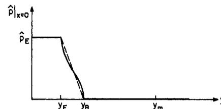
Fig. 2. Excess hole concentration  $\hat{p}$  at  $x = 0$  (along the junction edges and base surface). The dashed line is a first-order approximation for  $\hat{p}$  at the base surface.
