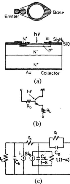
Fig. 1. p-i-n-transistor photodetector. (a) Structure. (b) Fundamental equivalent circuit. (c) Equivalent circuit in a common-collector configuration.
