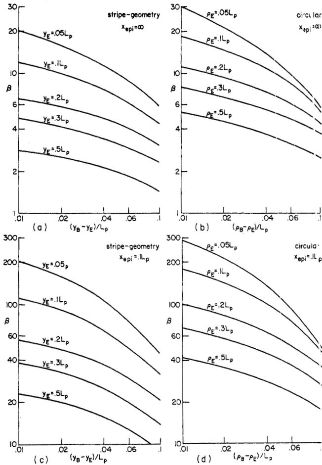
Fig. 3. Calculated current gain versus basewidth for various emitter widths. (a) Stripe geometry without a buried layer. (b) Circular device without a buried layer. (c) Stripe geometry with a buried layer ( $x_{epi} = 0.1 L_p$ ). (d) Circular device with a buried layer ( $x_{epi} = 0.1 L_p$ ).
