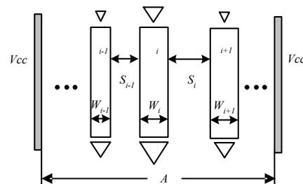
Figure 1. Structure of the bus wires
