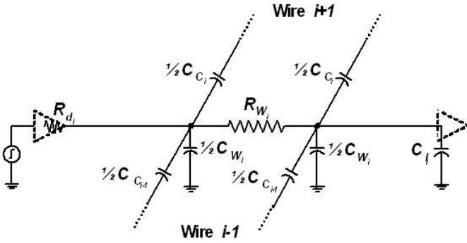
Figure 2. Equivalent circuit for calculating the  $i^{\text{th}}$  signal delay
